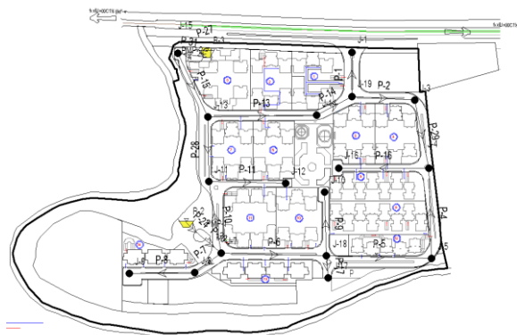
Fig4. Case B. loop network design using two hot water sources (PVC and galvanized pipe) (indicated with yellow color).
